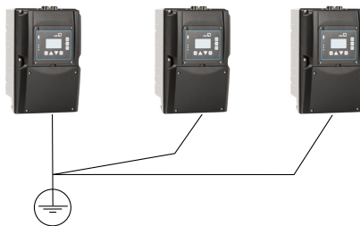
Fig. 24: Establishing an earth connection
